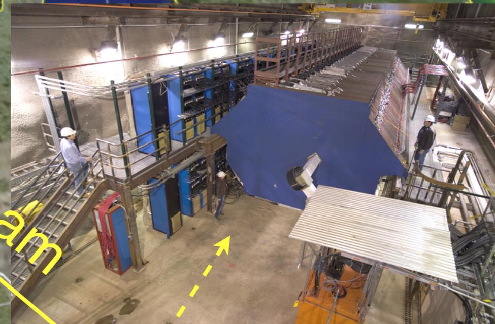
Both detectors are magnetized tracking calorimeters.
